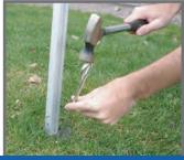
ALWAYS ANCHOR! To secure on grass or dirt, locate footplate, insert spike though hole, use hammer to drive spike. For hardpan anchoring; see website.
