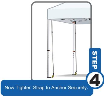
Repeat until all four Gravity-Stakes are secured.
